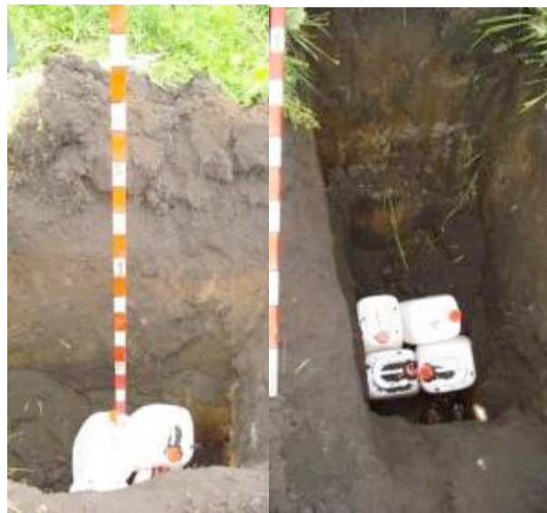
Fig. 19. Plastic cans (4 items). Size 35*25*20 cm. Deployment depth is 1.5 m.
