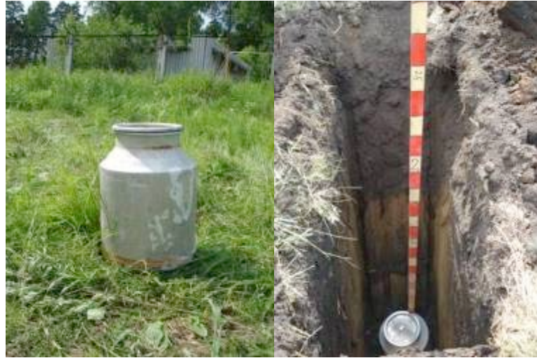
Fig. 22. Aluminum churn. D of the bottom part is 0.35 m, H= 0.5 m. Depth down to the lid is 2 m.
