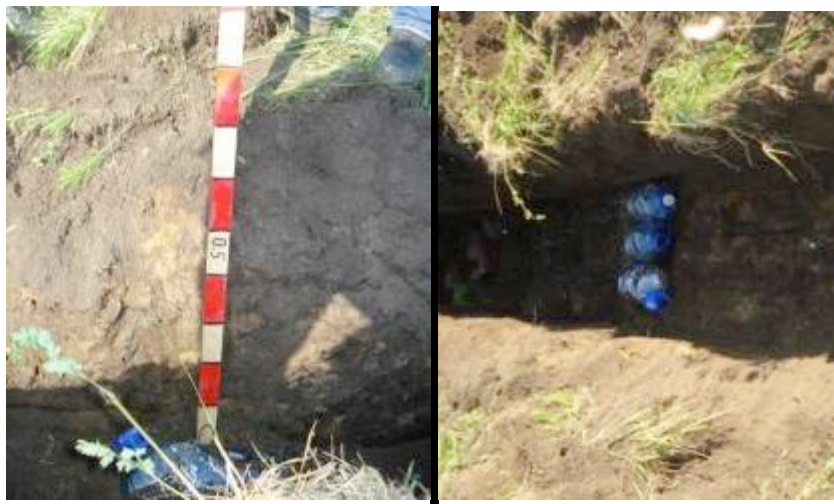
Fig. 5. Plastic bottle 1 item. (5 liters) with metallic shavings. Deployment depth is 0.8 m.
