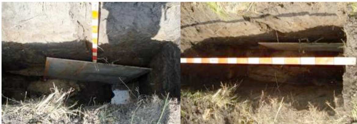
Fig. 12. Vertical iron sheet 1*1.25 m. The top edge reaches the depth of 1 m.
