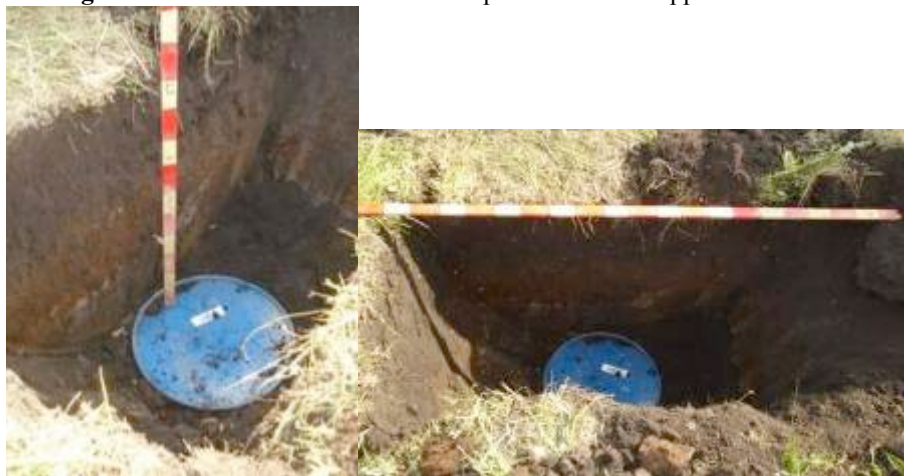
Fig. 31. Horizontal iron disk D=0.6 m. Deployment depth is 1 m
