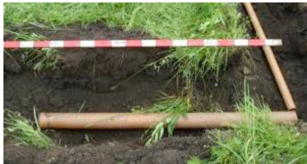
Fig. 1. Plastic tube with length 1.8 m, D= 110 mm. Deployment depth is 0.5 m.
