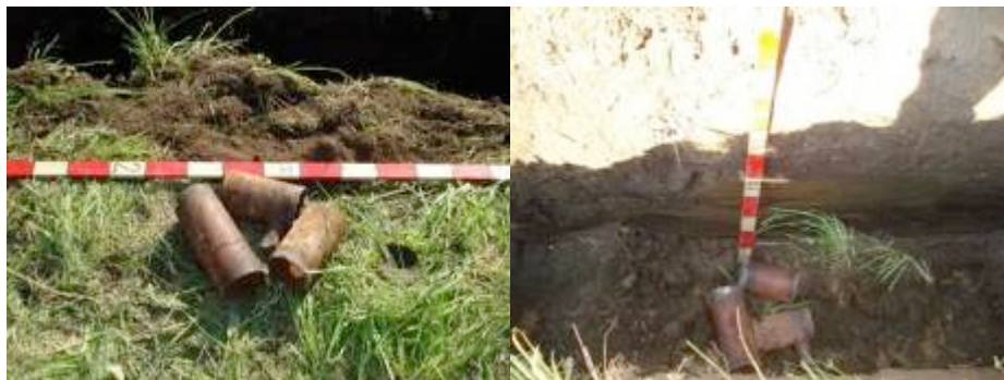
Fig. 6. Pieces of metal pipes (D 100 mm). The size of target 30*30 cm. Deployment depth is 1.1 m.
