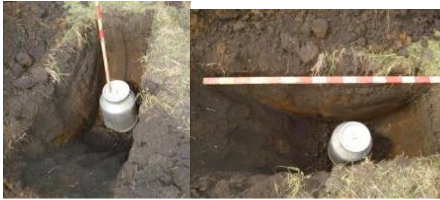
Fig. 21. Aluminum churn. D of bottom part is 0.35 m, H = 0.5 m. Depth down to the lid is 0.5 m.
