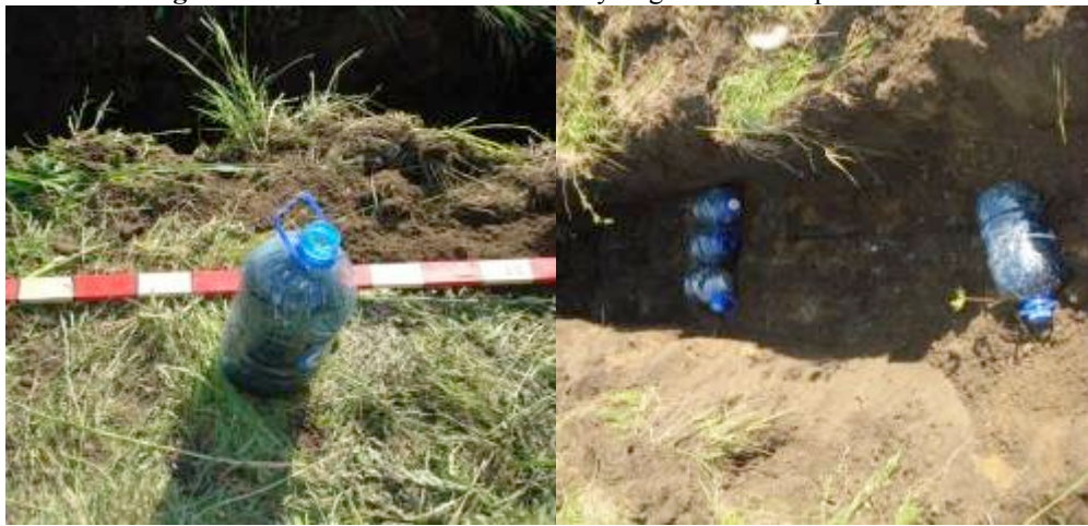
Fig. 4. Plastic bottle 1 item. (5 liters) with metallic shavings. Deployment depth is 0.5 m.
