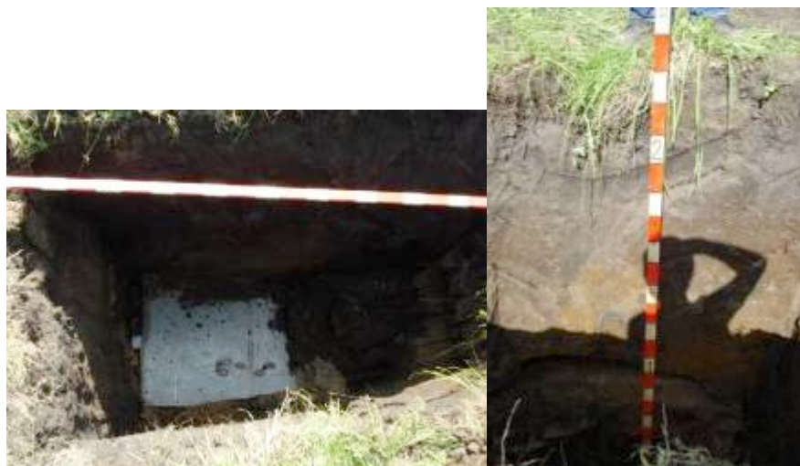
Fig. 11. Horizontal iron sheet 1 \times 1.25 m. Deployment depth is 2 m.
