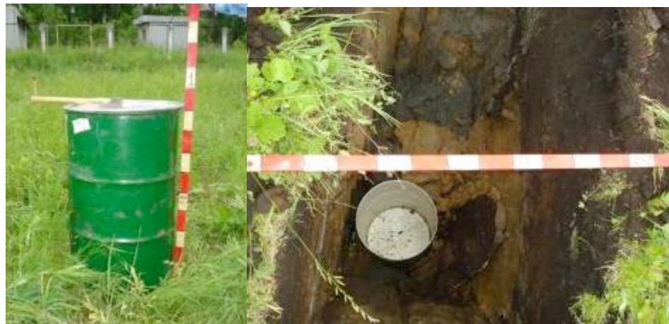
Fig. 23. Iron barrel. D= 0.56 m, H= 0.9 m. Depth down to the upper face is 0.9 m.
