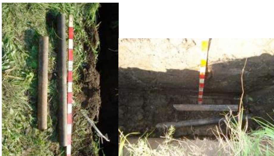
Fig. 7. «Antiaircraft projectiles». Pieces of round metallic bars with length 1.1 and 0.7 m, D= 7 cm. Piled side by side. Deployment depth is 1.5 m.
