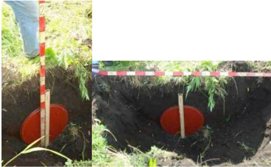
Fig. 30. Vertical iron disk D=0.6 m. Depth down to the upper face is 0.5 m.
