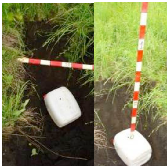
Fig. 17. Plastic can (1 item). Size 35*25*20 cm. Deployment depth is 0.5 m.
