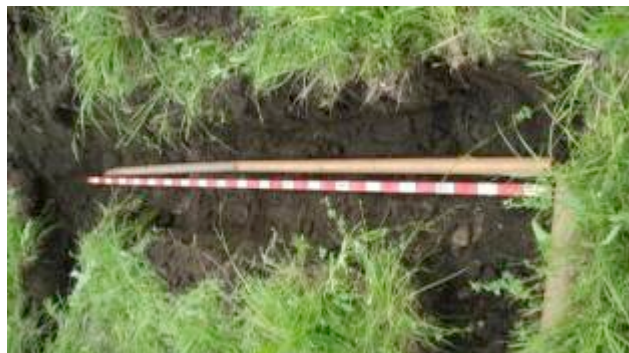
Fig. 2. Plastic tube with length 3.7 m, D= 60 mm. Deployment depth is 0.5 m.
