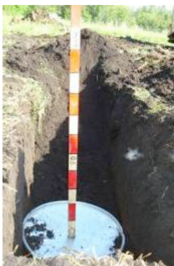
Fig. 10. Iron disk, D = 0.6 m. Deployment depth is 0.5 m.
