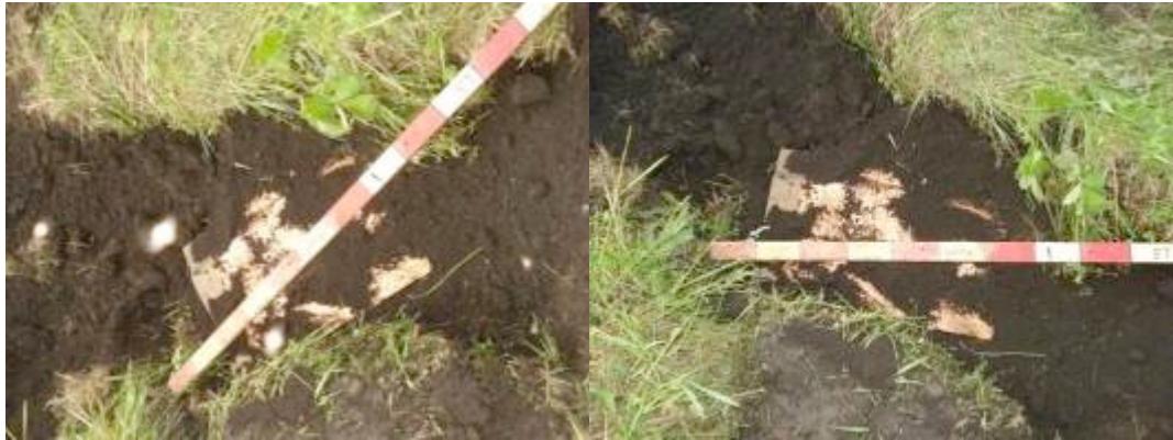
Fig. 27. Horizontal copper sheet 1*0.6 m tilted to axis. Deployment depth is 0.8 m.
