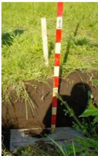
Fig. 8. Aluminum sheet 60*40 cm. Deployment depth is 0.5 m.
