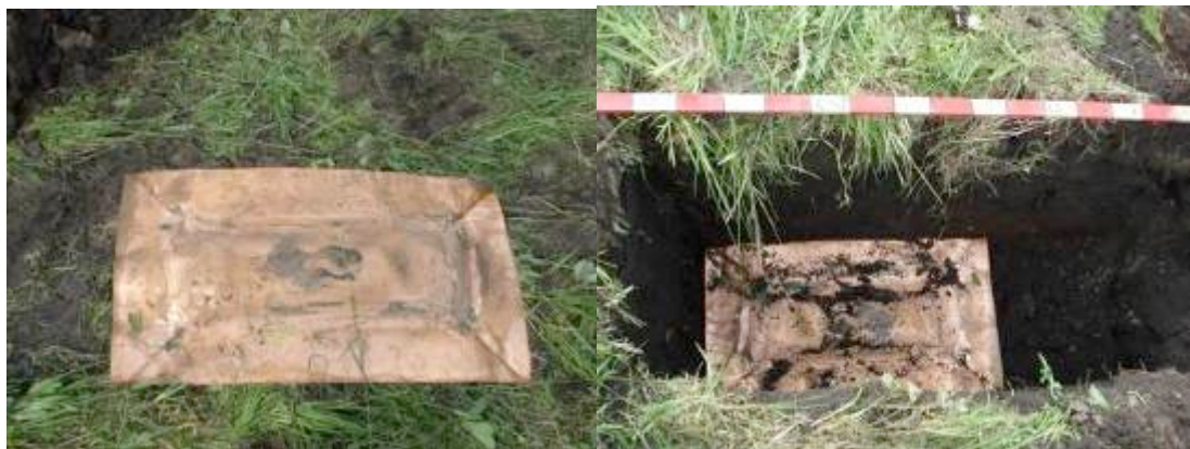
Fig. 29. Horizontal copper sheet 0.5*0.6 m.. Deployment depth is 0.2 m.
