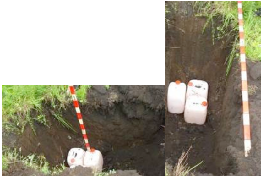
Fig. 18. Plastic can (3 items). Size 35*25*20cm. Deployment depth is 1 m.
