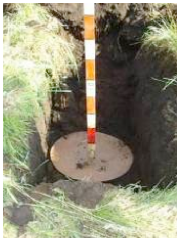
Fig. 9. Copper disk, D = 0.5 m. Deployment depth is 0.5 m.
